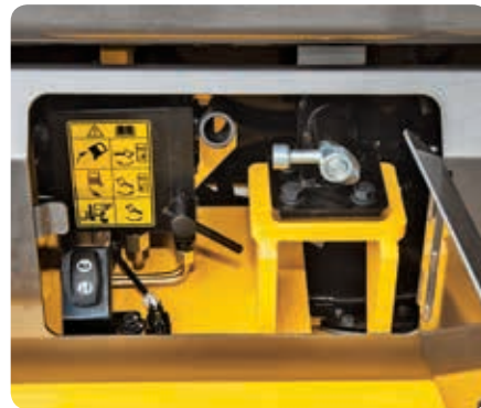
Cabin Tilting Automatic System Cabin tilting automatic system makes servicing of all power train components quick and easy. An electrically assisted hydraulic actuated cylinder tilts operator cabin to left side about 53 degrees for easy access to inside of truck components.
